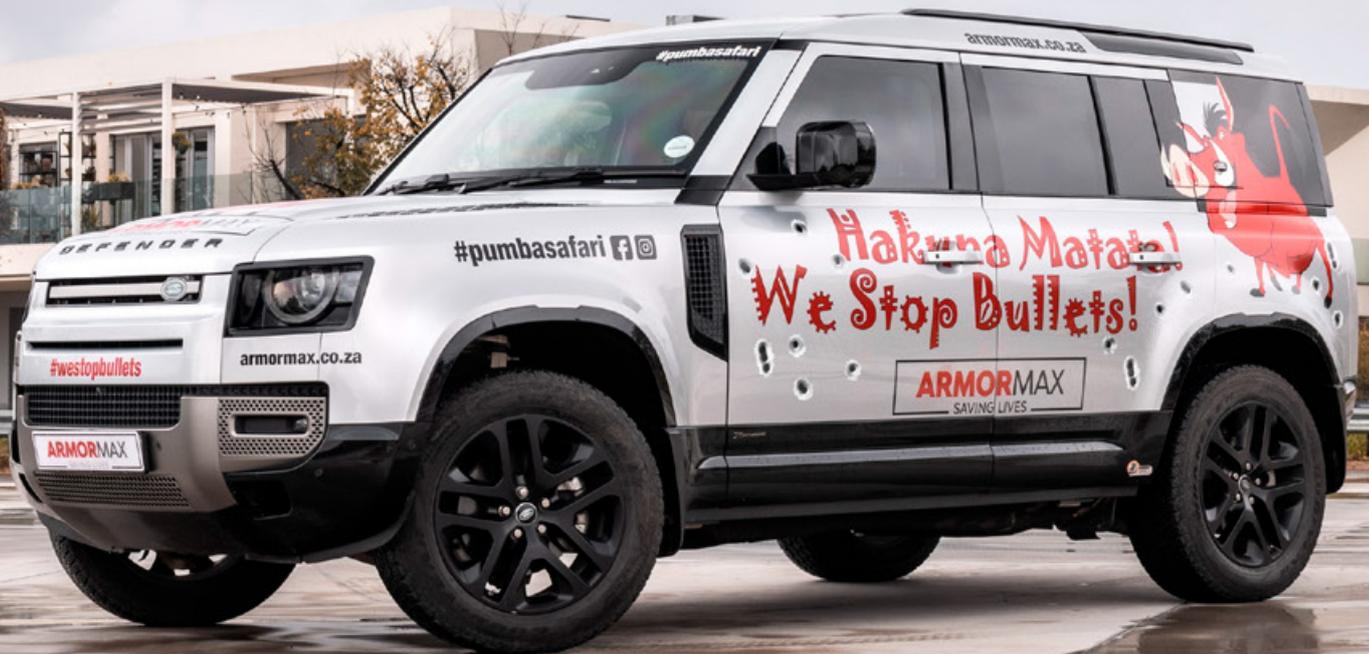
Armormax is proud to introduce it's new Land Rover Defender Armouring Package. Available in both B4 Handgun Protection and B6 Rifle Protection.
